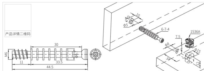
MKJSG-9-7 金属自攻牙 MKJSG-9-7 Metal self-driven screw
