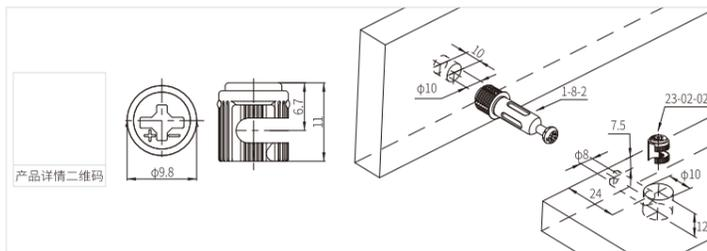
MKCAM-ZA-23-01-09 铁偏心轮 MKCAM-ZA-23-01-09 Iron eccentric cam
