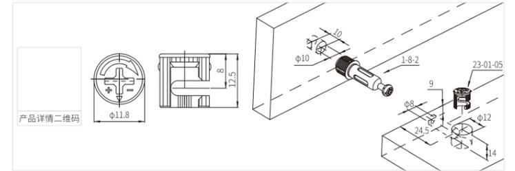
MKCAM-ZA-23-01-12 铁偏心轮 MKCAM-ZA-23-01-12 Iron eccentric cam
