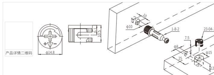
MKCAM-ZA-23-04-13 铁偏心轮 MKCAM-ZA-23-04-13 Iron eccentric cam
