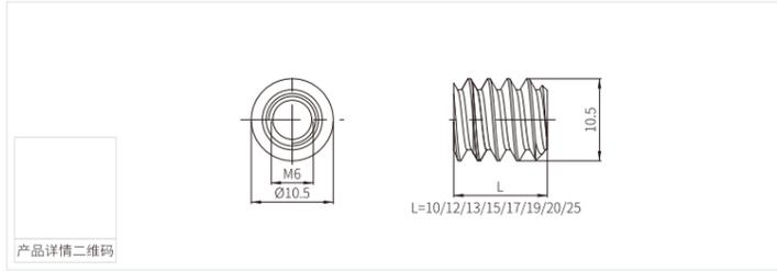
MK-CS-20-02-02 带介内外牙 MK-CS-20-02-02 Insert nut type D
