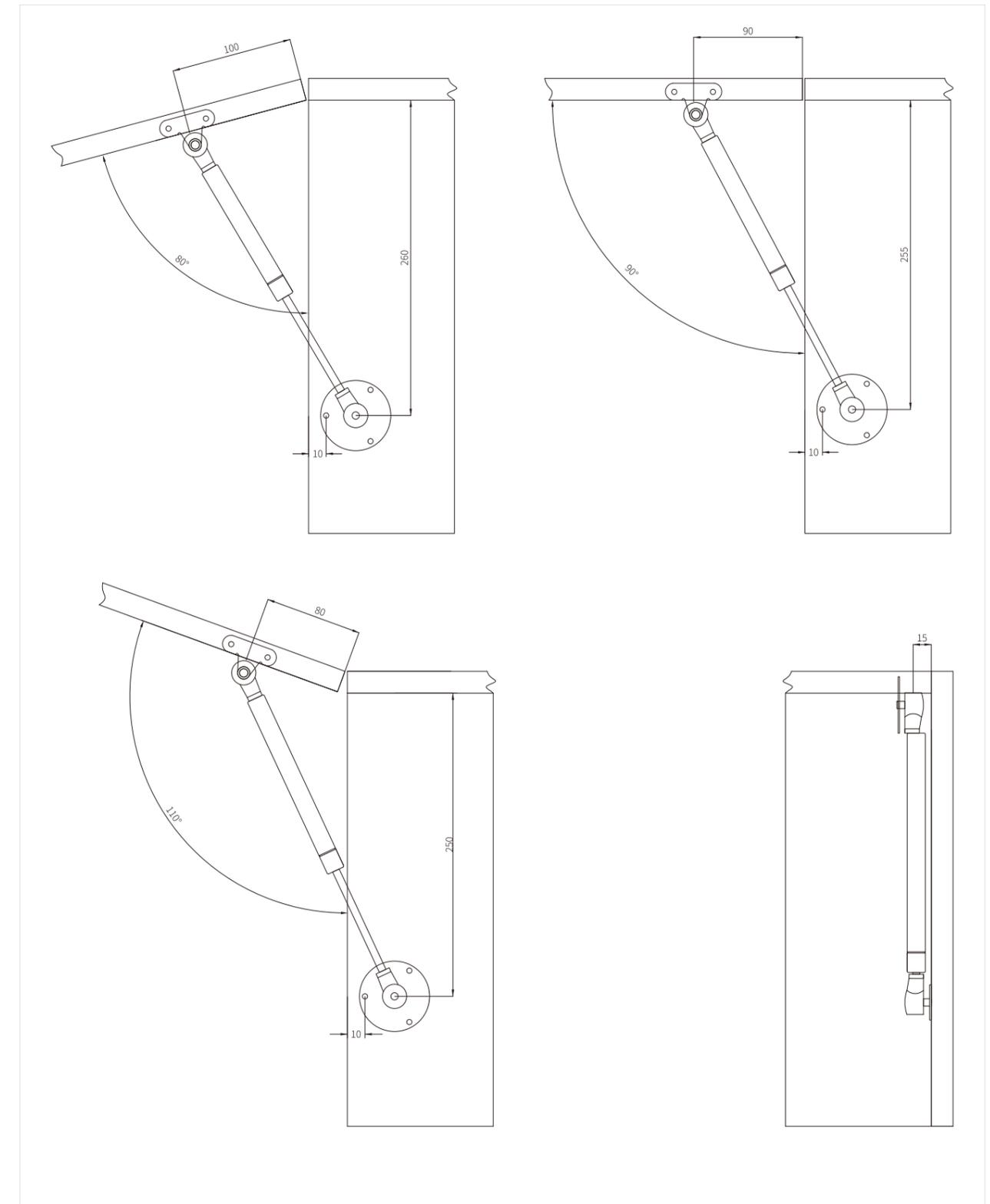
MK-KR-A002 铁头胶芯上翻支撑 MK-KR-A002 Lift up gas support with two steel fixators
