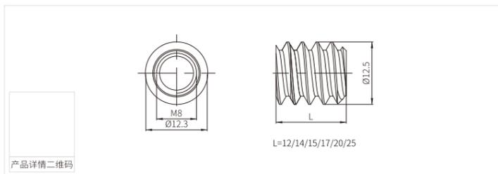
MK-铜膨胀螺母 MK-Copper expansion nut
