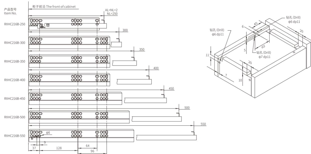
RX216B两节反弹隐藏滑轨(带插销) RX216B Two-segment Push-open Concealed Slide (with fixing pin)
