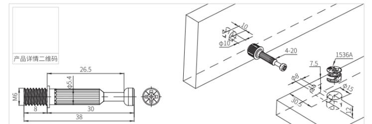
MK-JSG-4-22-1 金属竖纹杆 MK-JSG-4-22-1 Mental Bolt With Vertical Grain
