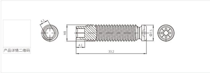
MK-M4 4厘沉头螺丝 MK-M4 Countersunk head bolt
