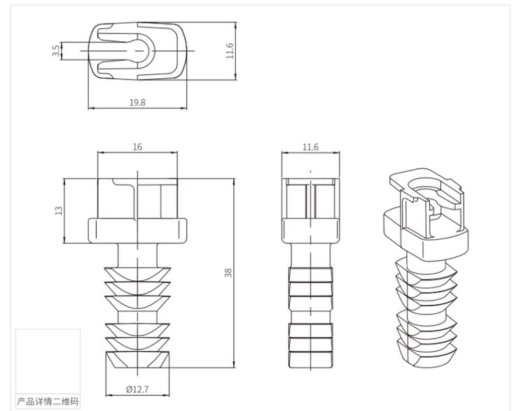
MK-SD-10厘4寸铁板托 MK-SD-10 4 inch iron shelf support
