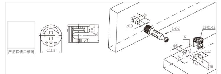
MKCAM-ZA-23-01-11 铁偏心轮 MKCAM-ZA-23-01-11 Iron eccentric cam
