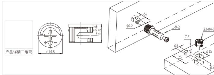
MKCAM-ZA-23-04-11 铁偏心轮 MKCAM-ZA-23-04-11 Iron eccentric cam
