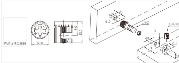
MKCAM-ZA-23-02-02 铁偏心轮 MKCAM-ZA-23-02-02 Iron eccentric cam
