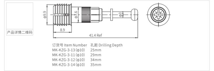
MK-KZG-3-11 快装一体杆 (φ8) MK-KZG-3-11 Spreading bolt
