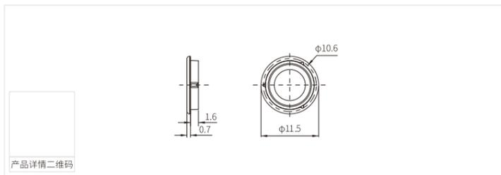
MK-KG-32-01-09 3# 12下沉式塑料盖 MK-KG-32-01-09 3# Countersunk plastic cover
