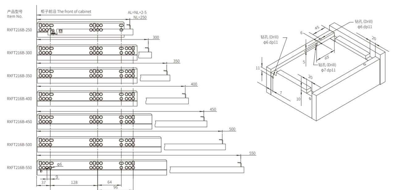
RX318三节缓冲隐藏滑轨(三维调节) RX318 Three-segment Soft-closing Concealed Slide (3D adjustment)
