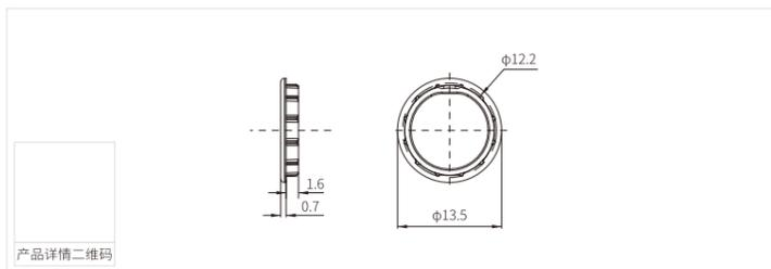
MK-KG-32-01-08 4# 10下沉式塑料盖 MK-KG-32-01-08 4# 10 Countersunk plastic cover
