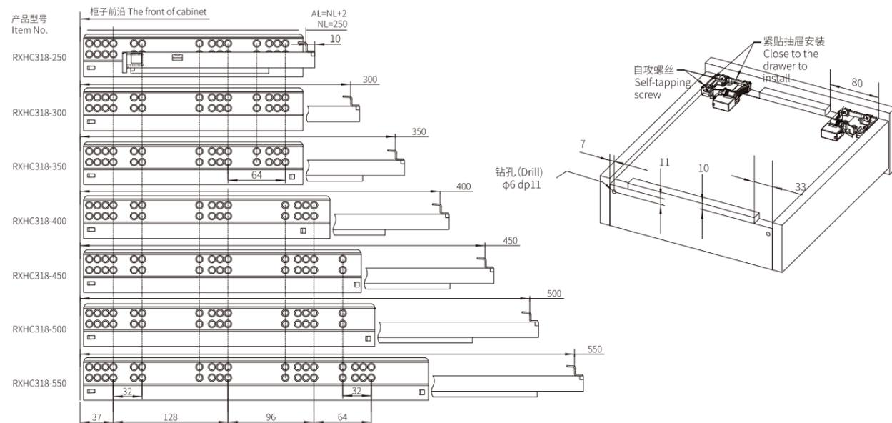
RX318三节反弹隐藏滑轨(三维调节) RX318 Three-segment Push-open Concealed Slide (3D adjustment)
