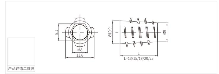
MK-ZA-51-61-12 无介内外牙螺母 MK-ZA-51-61-12 Insert nut type E
