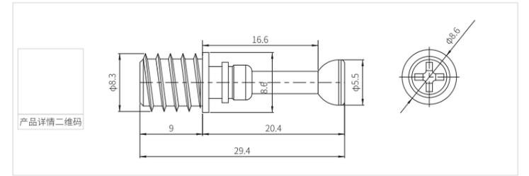
MK-JSG-4-20 金属竖纹杆 MK-JSG-4-20 Mental Bolt With Vertical Grain
