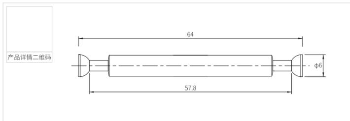
MK-KZG-3-11 快装一体杆 (φ10) MK-KZG-3-11 Spreading bolt
