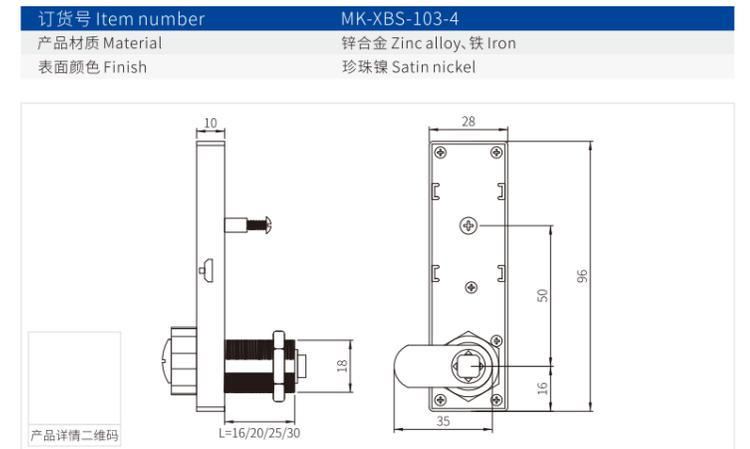
MK-CLW-三联锁 MK-CLW-三联锁 MK-CLW-Three linkage lock
