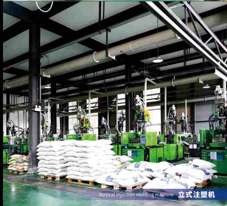
Vertical injection molding machine 立式注塑机
