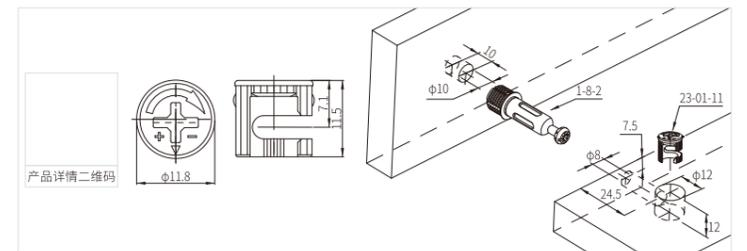
MKCAM-ZA-23-04-07 铁偏心轮 MKCAM-ZA-23-04-07 Iron eccentric cam
