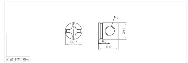
MK-ZA-51-86-17 带介内外牙螺母 MK-ZA-51-86-17 Insert nut type D
