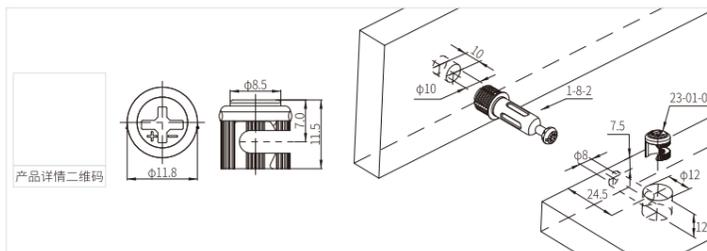
MKCAM-ZA-23-01-05 铁偏心轮 MKCAM-ZA-23-01-05 Iron eccentric cam
