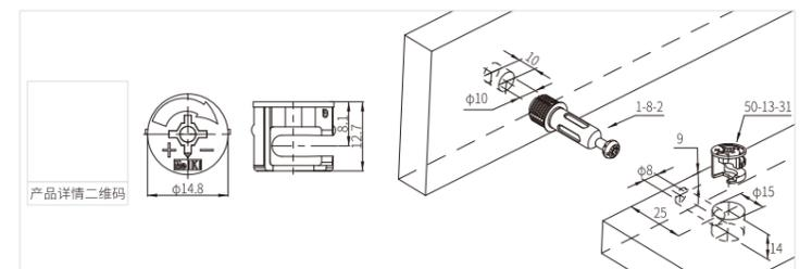
MKCAM-ZA-23-02-01 铁偏心轮 MKCAM-ZA-23-02-01 Iron eccentric cam
