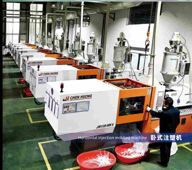
Horizontal injection molding machine 卧式注塑机
