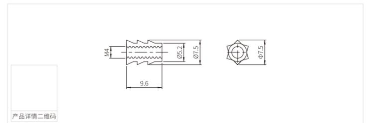
MK-ZA-51-65-12 带介内外牙螺母 MK-ZA-51-65-12 Insert nut type D
